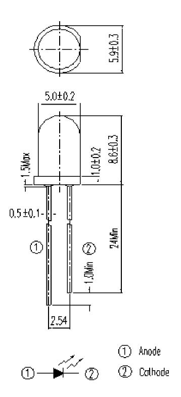
Note: Tolerances unless dimensions ±0.25mm
