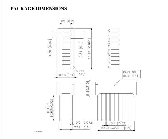
NOTES: 1. All dimensions are in millimeters. Tolerances are  $\pm$  0.25 mm unless otherwise note. 2. Pin tip's shift tolerance is  $\pm$  0.4 mm.
