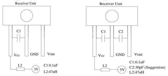
Note: For having good coupling, the C1,C2 capacitor must be placed within 7mm
