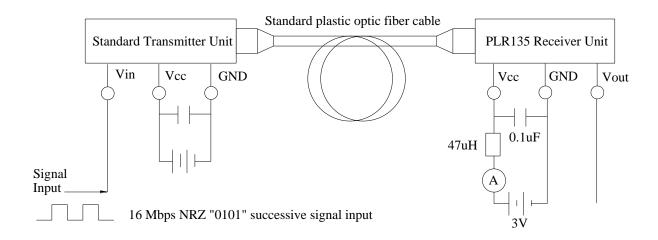
\*Fig.3 Measuring Method of Output Voltage, Pulse and Jitter
