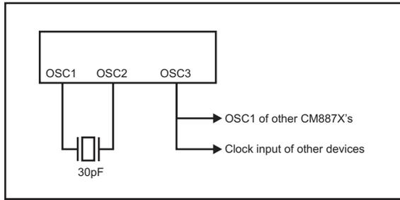
Figure 7. CM8870C Crystal Connection (PLCC Package Only)
