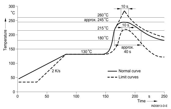
Pb-free solder material (based on JEDEC J-STD 020C)
